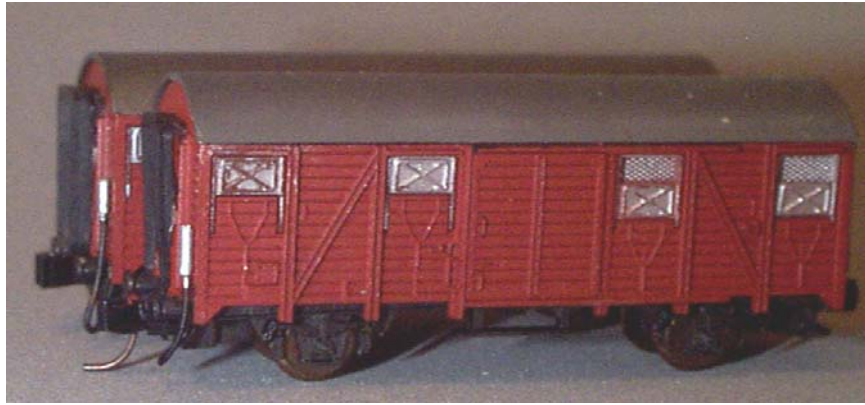
Figure 2 - Comparison of Retracted (foreground) and Extended Diaphragm
